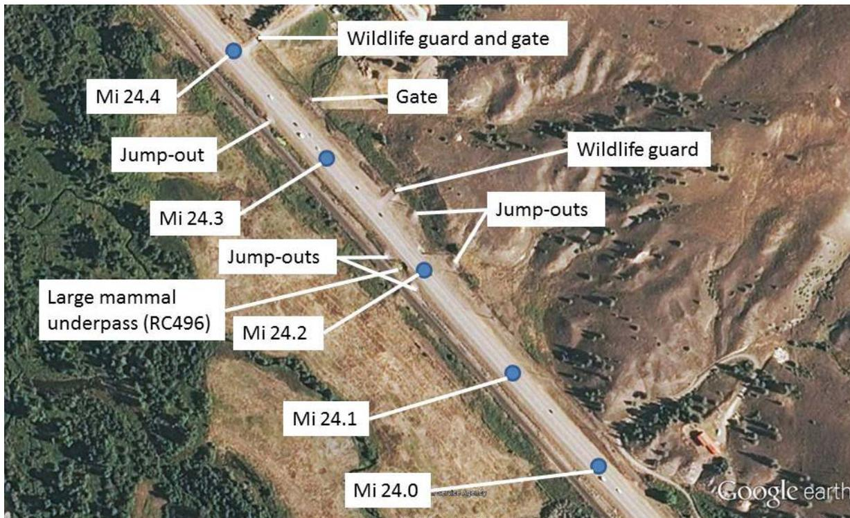
Figure 15: The mile markers, large mammal underpass, wildlife guards, gates and jump-outs between mi marker 24.0-24.4 at the potential concentration of large mammal-vehicle collisions in the Ravalli Curves area. Note that there is a wildlife fence in this area on both sides of the road that ties together the large mammal underpass, the jump-outs, and the wildlife guards and gates.
